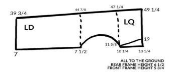
The maximum combined length of door and quarter together, front to back, is as follows:
